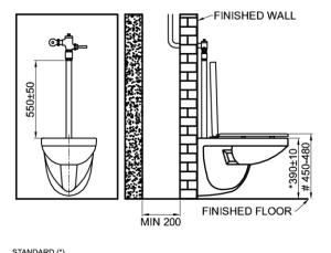
STANDARD (\*) 390±10 from floor finishing to the rim of water closet HANDICAPPED (#) 450-480 from floor finishing to the top of the water closet seat
