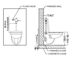
STANDARD (\*) - 390±10 from floor finishing to the rim of water closet.  $\begin{array}{l} \mbox{HANDICAPPED (\#)} - 450 \sim 480 \mbox{ from floor finishing to the top of the water closet seat.} \\ 750 \mbox{ from the front edge of the water closet to the rear wall.} \end{array}$
